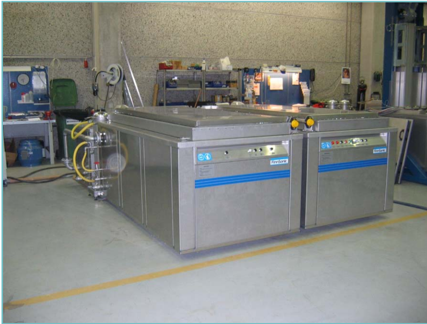
Ultrasonic cleaning system for drill pipes Client: NAM, the Netherlands
