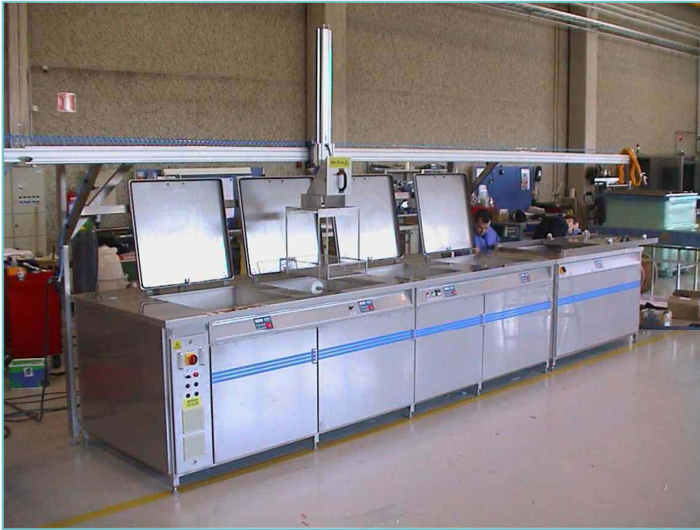
Ultrasonic cleaning system for valves and pipe parts Client: Halliburton Energy Services, Brazil
