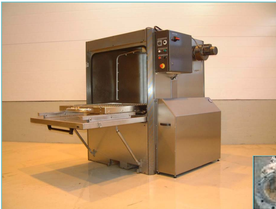
Spray cleaner for gate valves Client: Sperry Drilling Services, Mexico
