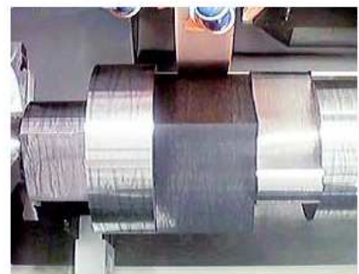
Pendulum Grinding of square component
