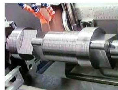
Pendulum-grinding of three-edged component
