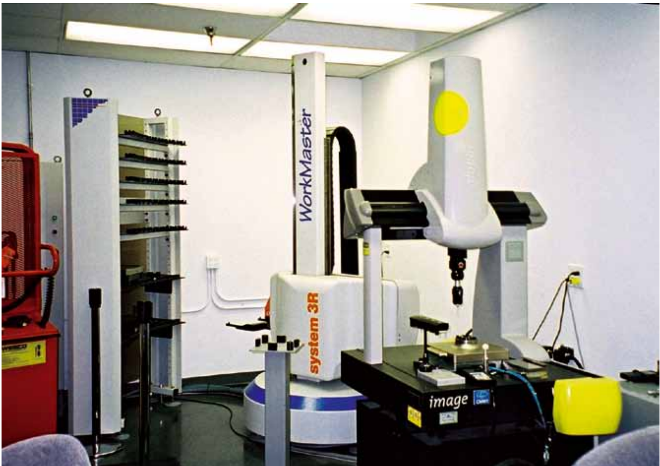
The Brown & Sharp CMM is also benefiting from 3R automation
