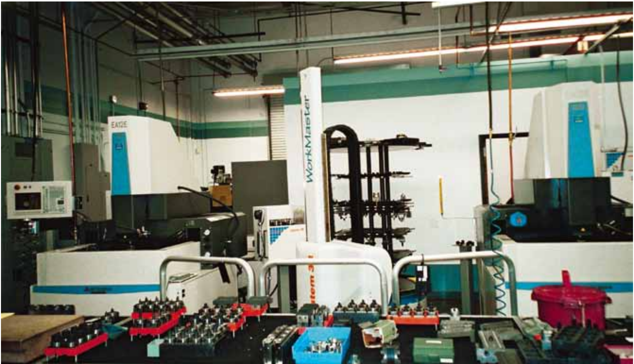
The WorkMaster serves two Mitsubishi sinkers, operating 24/7
